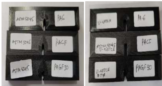
Fig. 6: Test Specimens U and V Notch
