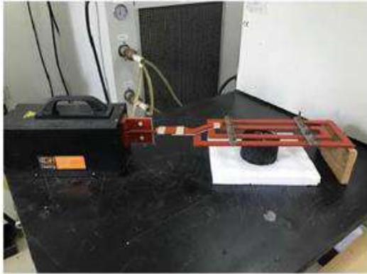
Fig. 2: Induction heating in laboratory
